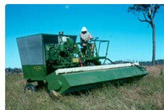
Harvesting seed with brush harvester
